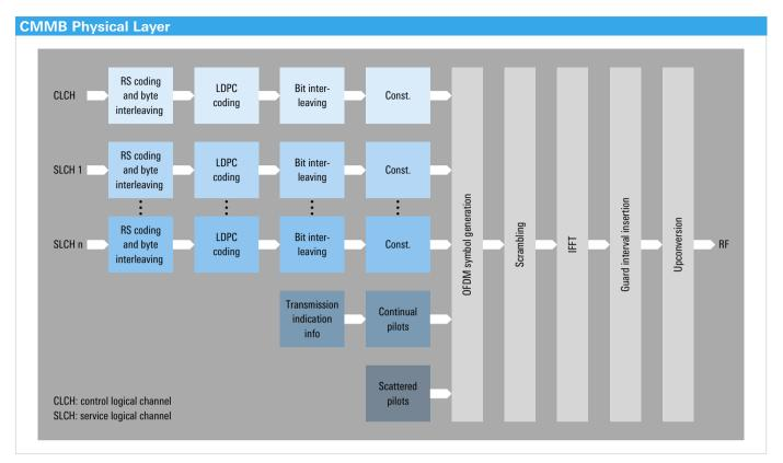
FIG 3 CMMB physical layer with logical channels.
