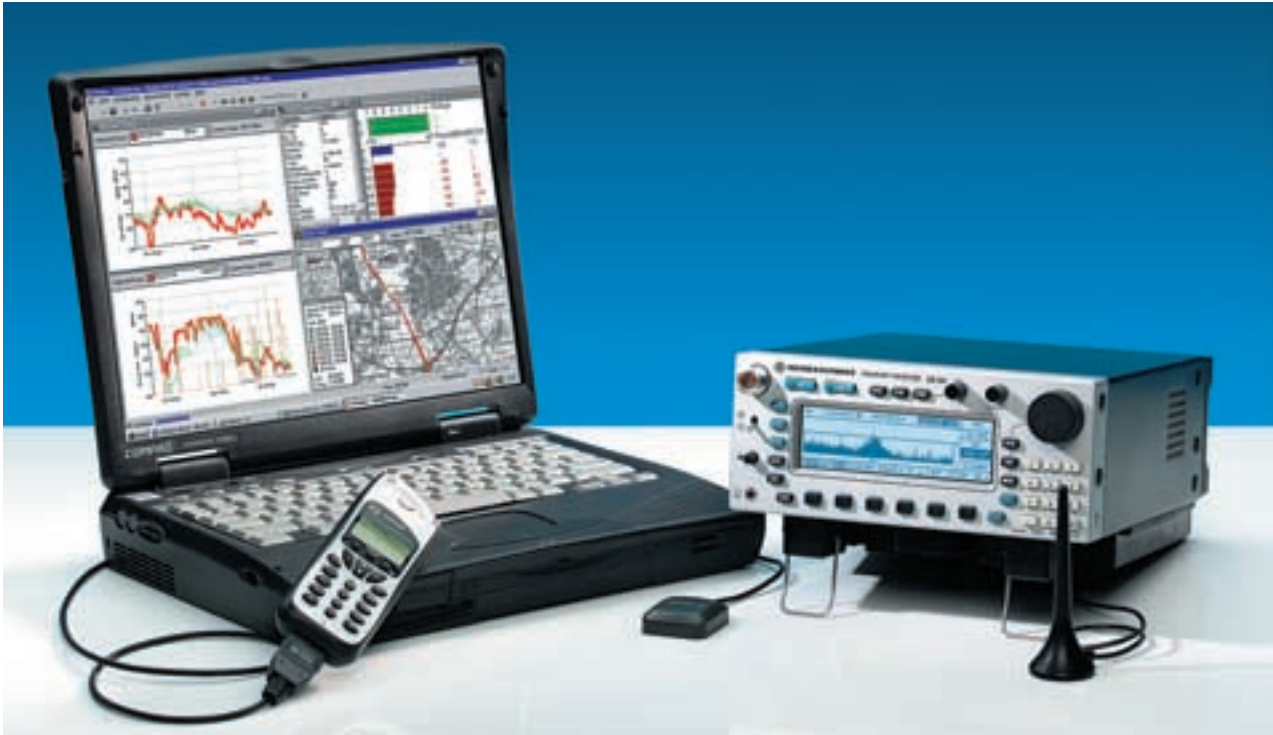
FIG 1 EB 200 is ideally suited for indoor coverage measurements and mobile applications in vehicles
