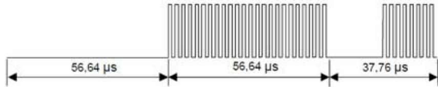
Figure 14: Start of frame when using one subcarrier
