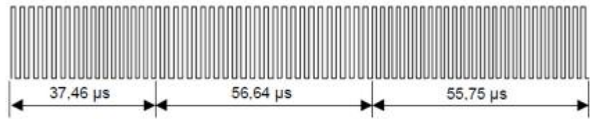
Figure 17: End of frame when using 2 subcarriers
