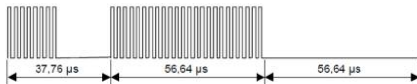
Figure 16: End of frame when using one subcarrier
